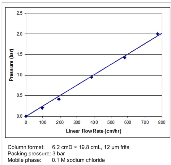
Figure 1 Pressure-flow properties of POROS™ XS resin
