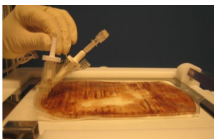
Figure 13 Flush Dynabeads™ magnetic beads from the outlet ports
